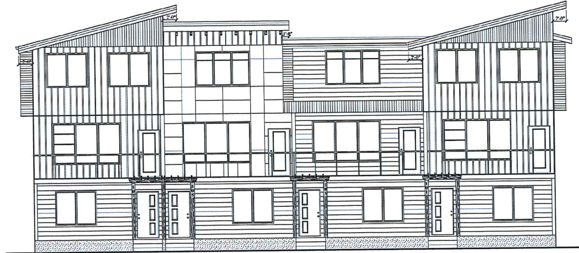
FRONT ELEVATION - KERRISDALE ROAD
