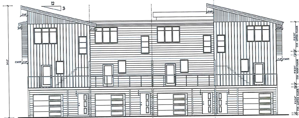
REAR ELEVATION - INTERIOR LANE
